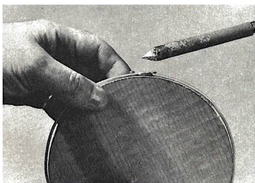
To make a fruit basket, use a 7-inch wood disc as a template for forming and soldering the stiff wire frame. Right—After soldering the screen bottom to the wire ring, trim away the excess with tin snips.
