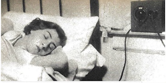
Left—The outfit set up so that the wire is around an open window, thereby awakening the sleeping person if anyone attempts to enter the room. It can also be used in a gas station to notify the attendant when a car pulls in.
