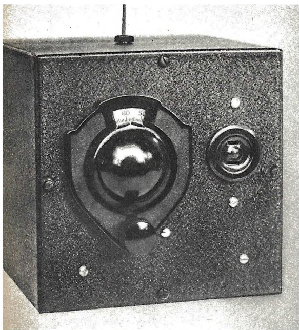
A front view of the completed relay. The dial controls the sensitivity of the magic wire. The socket mounted on the right side of the panel is for the plug connected to the alarm bell or light actuated by the relay. At the right is shown an inside view with the cabinet removed.
