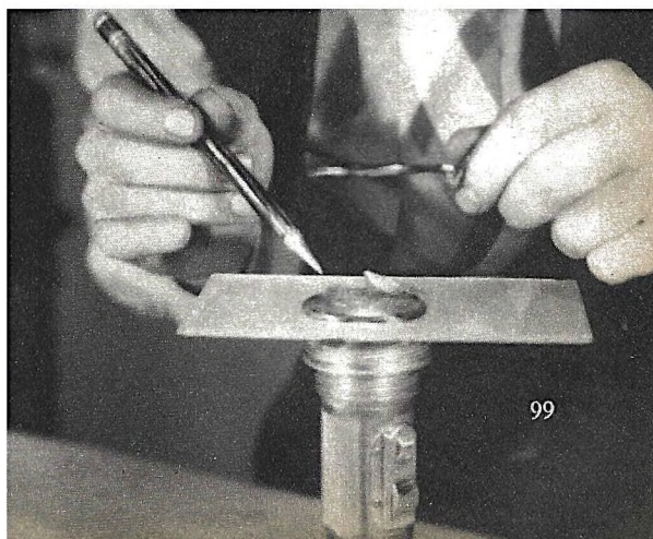
Above is shown the microscope in use after it is equipped with Polaroid. Below is shown a simple method of inspecting Cellophane under polarized light. A flashlight is stood on end, a piece of ground glass is placed on top of it, and Polaroid is placed on top of this. Commonplace materials often take on brilliant colors when subjected to polarized light.
