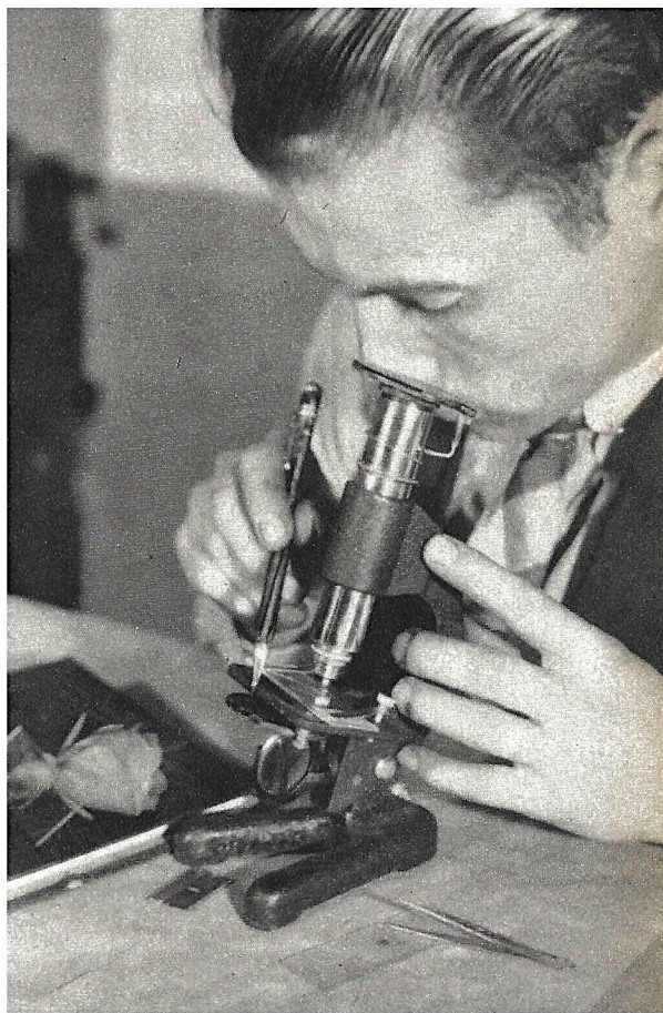
Above is shown the microscope in use after it is equipped with Polaroid. Below is shown a simple method of inspecting Cellophane under polarized light. A flashlight is stood on end, a piece of ground glass is placed on top of it, and Polaroid is placed on top of this. Commonplace materials often take on brilliant colors when subjected to polarized light.
